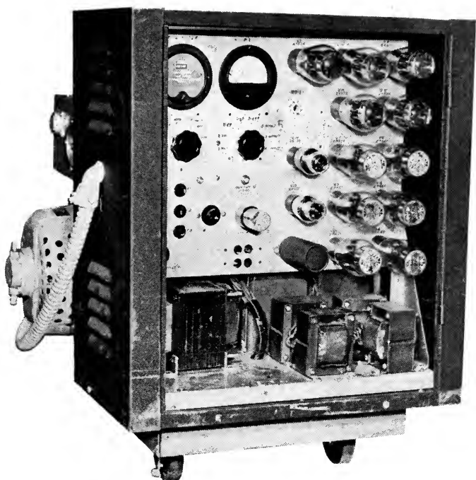
Fig. 41. Frequency converter and power supply regulator.
